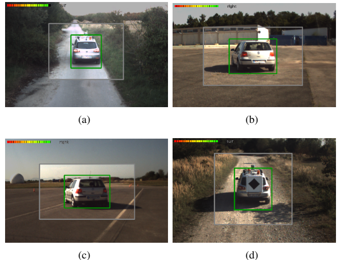
Fig. 6: Template-based Tracking: (a-c) with vehicle-specific model. (d) based on generic model.
