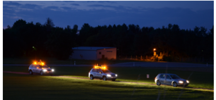
Fig. 1: Autonomous convoy driving at night. A VW Touareg following a VW Tiguan which follows a manually-driven VW Golf. Orange lights indicate an activated autonomous mode.
