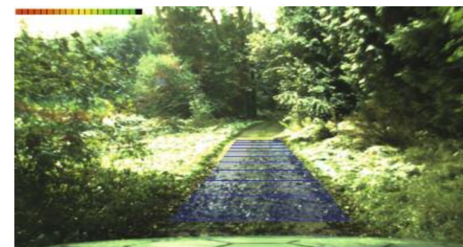
Fig. 3: Visually recognised dirt road in unstructured terrain and indication of the recognition quality
