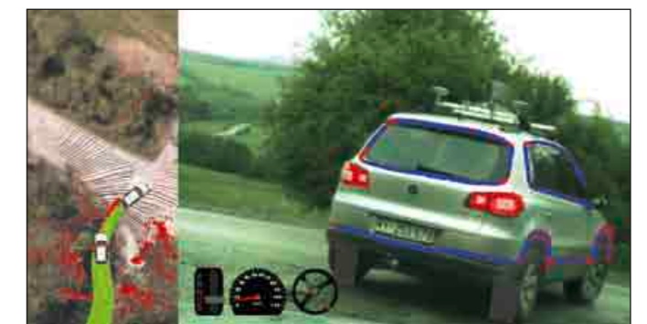
Fig. 4: In the left part, the path is shown which the UGV has to follow. Green circles represent local waypoints and their probabilistic uncertainty. Additionally, obstacle information (red dots) are shown superimposed on a georeferenced aerial image. The right part shows the colour camera image with an overlay of the estimated model position
