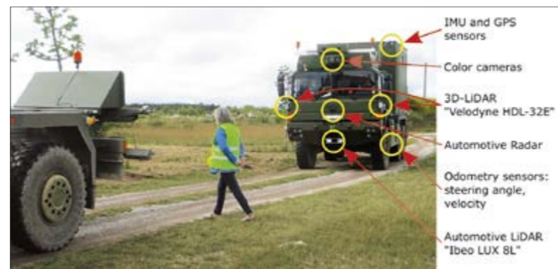
Fig. 2: TULF ("Technologieträger unbemanntes Landfahrzeug", or Unmanned Land Vehicle Technology Demonstrator) stops in front of a dynamic obstacle during the convoy scenario. The sensors used for automated following are labeled
